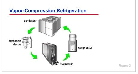
The purpose of the compressor in a refrigeration system is to raise the pressure of the refrigerant vapor from evaporator pressure to condensing pressure. It delivers the refrigerant vapor to the condenser at a pressure and temperature at which the condensing process can be readily accomplished, at the temperature of the air or other fluid used for condensing.
